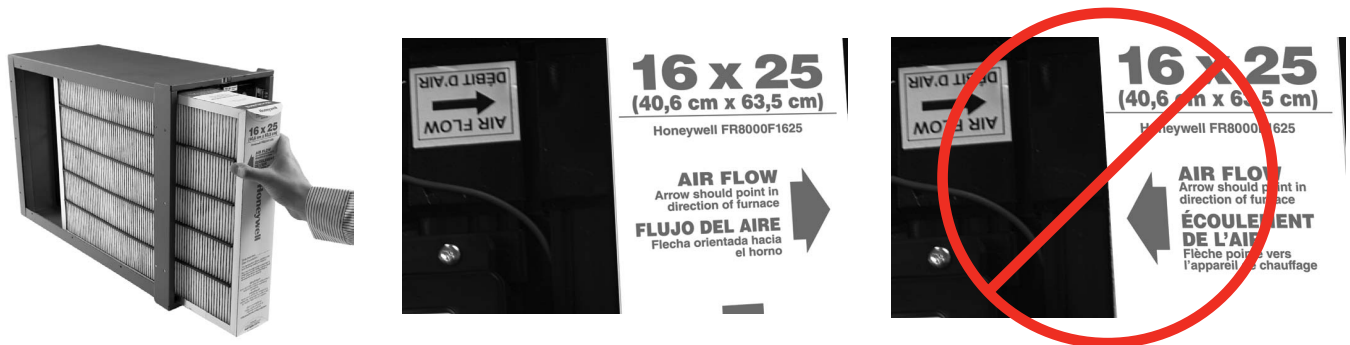
Fig. 18: Make sure that the arrows on the filter point in the same direction as the arrow on the enhancement module. This will be in the same direction as airflow.
