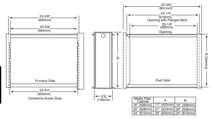
NOTE: Media cabinet is matched to the bottom opening on furnace. May also be used for side return.
