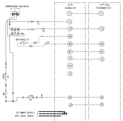
A/C RECTIFIER ACR FAN CAPACITOR CN WIRECONNECTOR COMPRESSOR RUN CAPACITOR STARTING CAPACITOR cs CAPACITOR SWITCHING RELAY INDOOR FAN RELAY нрсо HIGH PRESSURE CUTOUT SWITCH INTERNAL OVERLOAD PROTECTOR LPCO LOW PRESSURE CUTOUT SWITCH SYSTEM ON-OFF SWITCH MS COMPRESSOR MOTOR CONTACTOR OUTDOOR ANTICIPATOR OUTDOOR FAN THERMOSTAT OUTDOOR TEMPERATURE SENSOR ODS OUTDOOR THERMOSTAT SWITCH OVER VALVE SOLENOID DISCHARGE LINE THERMOSTAT TIME DELAY RELAY(5 SEC DELAY ON)
