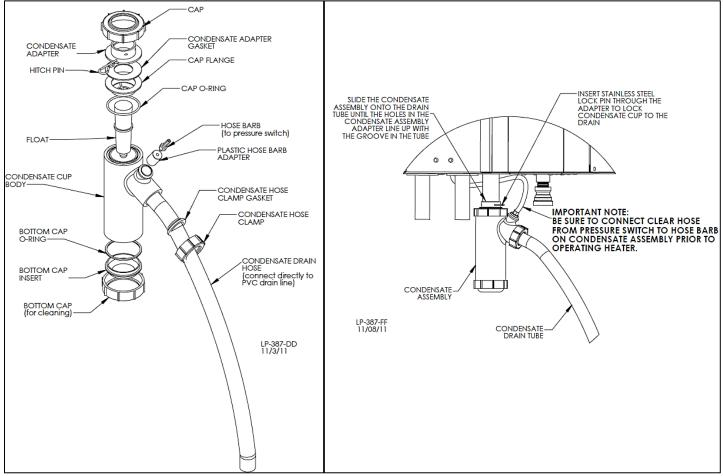
Figure 15-1 - Condensate Detail, 15-2 – Condensate Trap Installation
