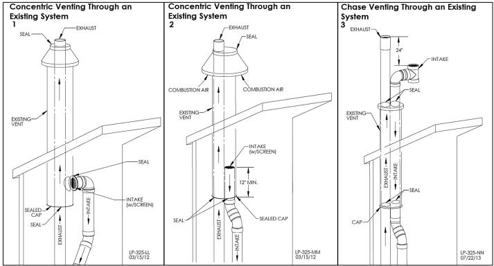
Figures 24 – 1, 24 – 2 Concentric Venting Through an Existing System, 24 – 3 Chase Venting Through an Existing System NOTE: This drawing is meant to demonstrate system venting only. The installer is responsible for all equipment and detailing required by local codes.
