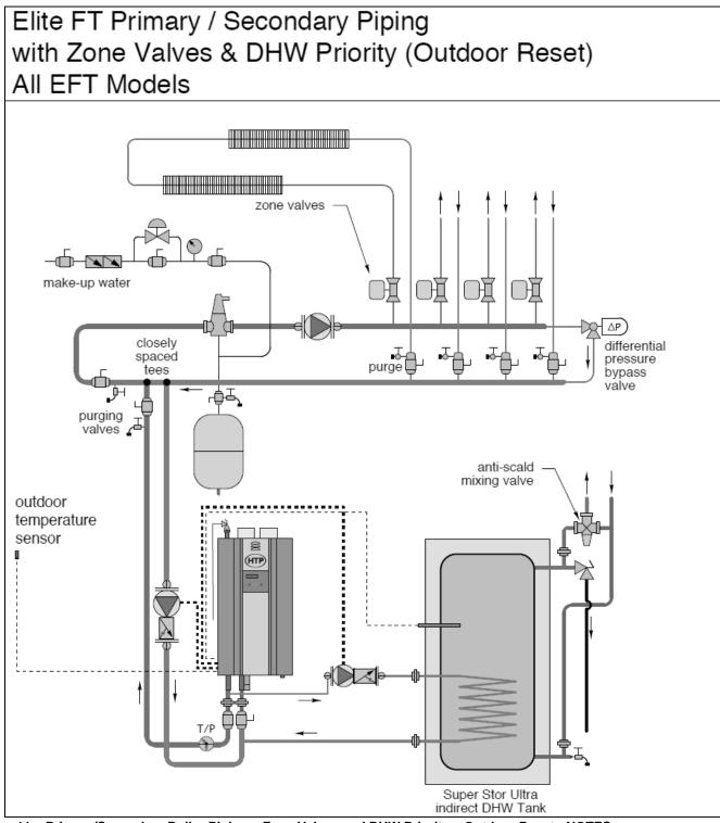
Figure 11 – Primary/Secondary Boiler Piping – Zone Valves and DHW Priority – Outdoor Reset - NOTES:
