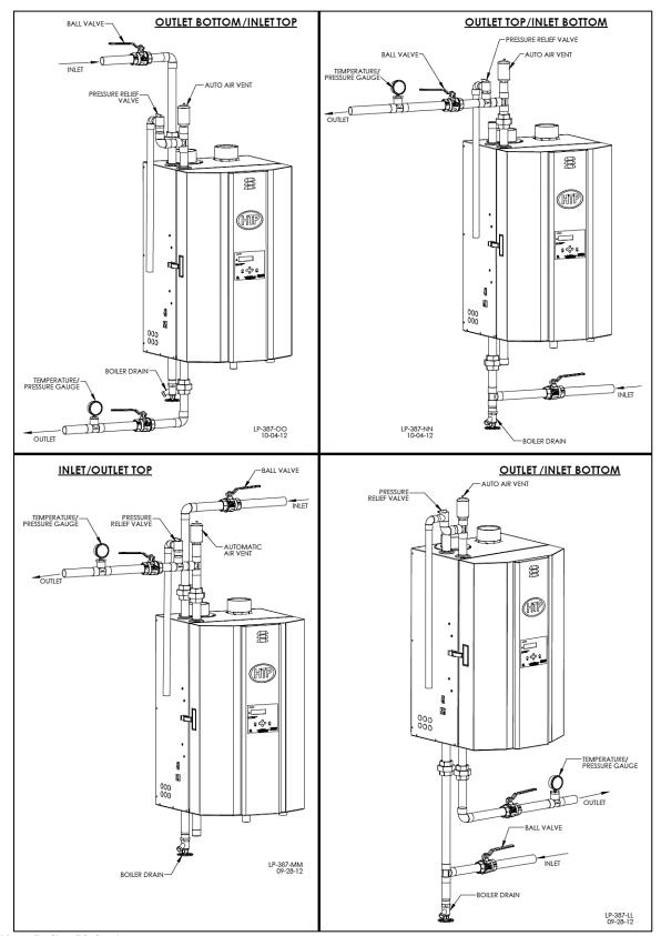
Figure 7 – Near Boiler Piping\* – NOTE: This drawing is meant to show system piping concept only. Installer is responsible for all equipment and detailing required by local codes. \*Top / Bottom Supply / Return Connections available on EFT-155, EFT-199, EFT-285, and EFT-399 Models ONLY
