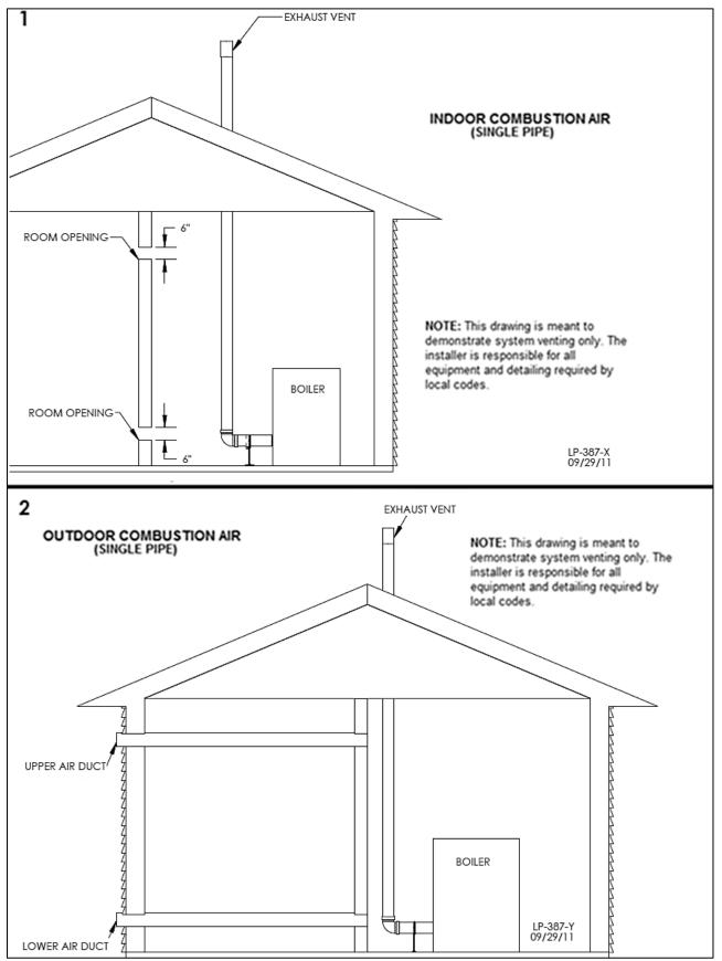
Figure 26 – 1, 26 - 2 NOTE: These drawings are meant to demonstrate system venting only. The installer is responsible for all equipment and detailing required by local codes.
