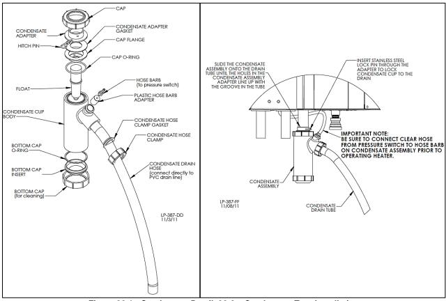
Figure 36-1 - Condensate Detail, 36-2 - Condensate Trap Installation
