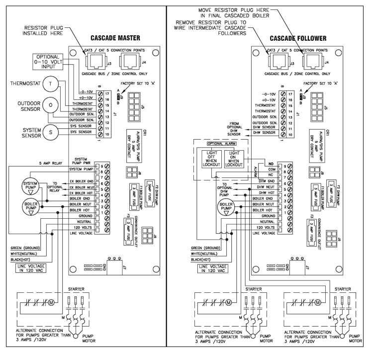
Figure 33 – Cascade Master and Follower Wiring
