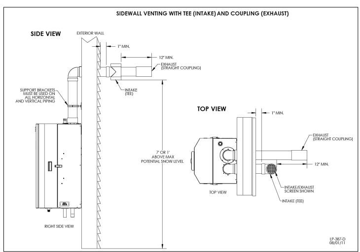
Figure 19 – Sidewall Venting with Tee (Intake) and Coupling (Exhaust) (Standard Equipment) NOTE: Drawing is meant to demonstrate system venting ONLY.
