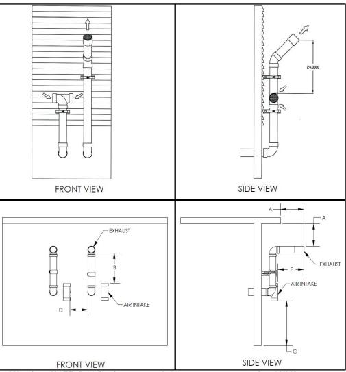
Figure 23 – Horizontal Venting - NOTE: Drawing is meant to demonstrate system venting ONLY.
