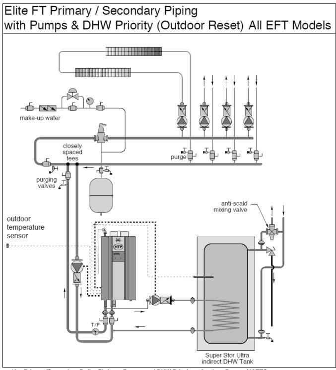
Figure 12 – Primary/Secondary Boiler Piping – Pumps and DHW Priority – Outdoor Reset - NOTES:
