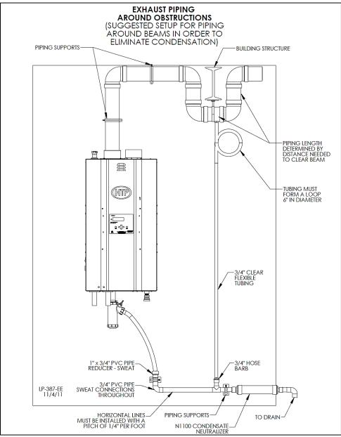
Figure 17 – Piping Exhaust around Obstructions – Suggested Condensate Removal
