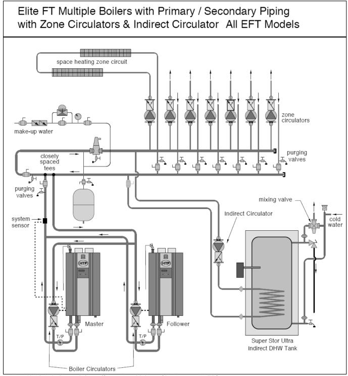
Figure 13 – Multiple Boilers – Primary/Secondary Piping – Circulators - NOTES:
