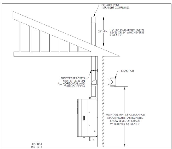
Figure 22 – Unbalanced Flue/Vertical Vent - NOTE: Drawing is meant to demonstrate system venting ONLY.
