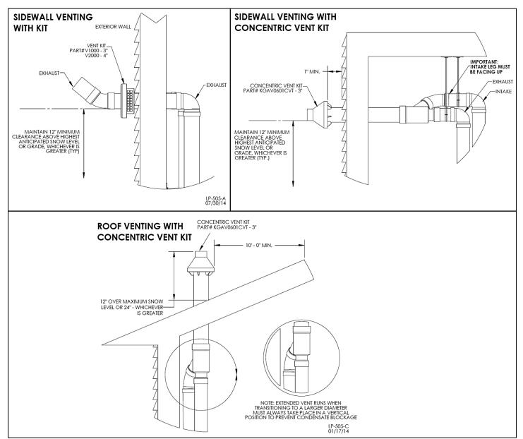
Figure 20 – Venting with Optional Kits (NOT INCLUDED WITH THE WATER HEATER) NOTE: These drawings are meant to demonstrate system venting only. The installer is responsible for all equipment and detailing required by local codes.
