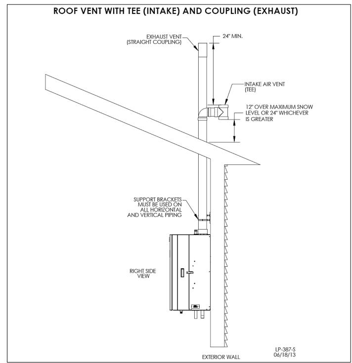
Figure 21 – Roof Vent with Tee (Intake) and Coupling (Exhaust) - NOTE: Drawing is meant to demonstrate system venting ONLY.
