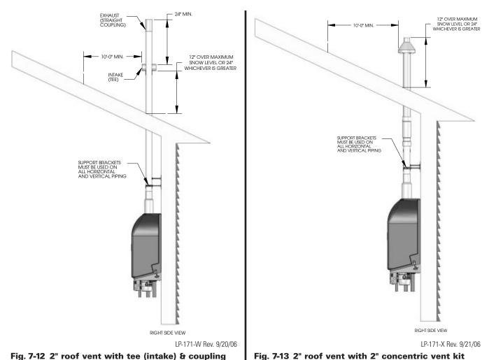
NOTE: When placing support brackets on vent piping, the first bracket must be within 1 foot of the appliance and the balance at 4 foot invervals on the vent pipe. The heater venting must be readily accessible for visual inspection for the first three feet from the heater.
