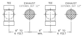
Fig. 7-2 Multiple Vent Spacing\*
