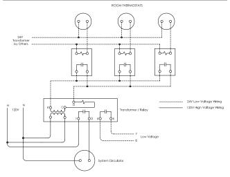
SECONDARY SYSTEM CIRCULATOR WIRING
