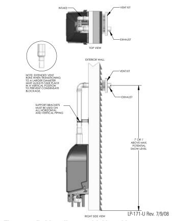
Fig. 7-10 2" sidewall vent with V500 kit
