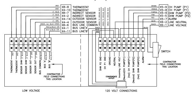
Munchkin Contender Internal Wiring Diagram
