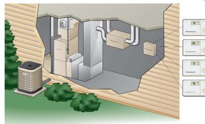
Since heat rises, homes with multi-levels benefit greatly from zoning. Zone controls divide the home into individual spaces, each with their own thermostat. When the thermostat within a zone reaches its desired level the damper to that zone is shut down, thereby eliminating vast temperature differences.
