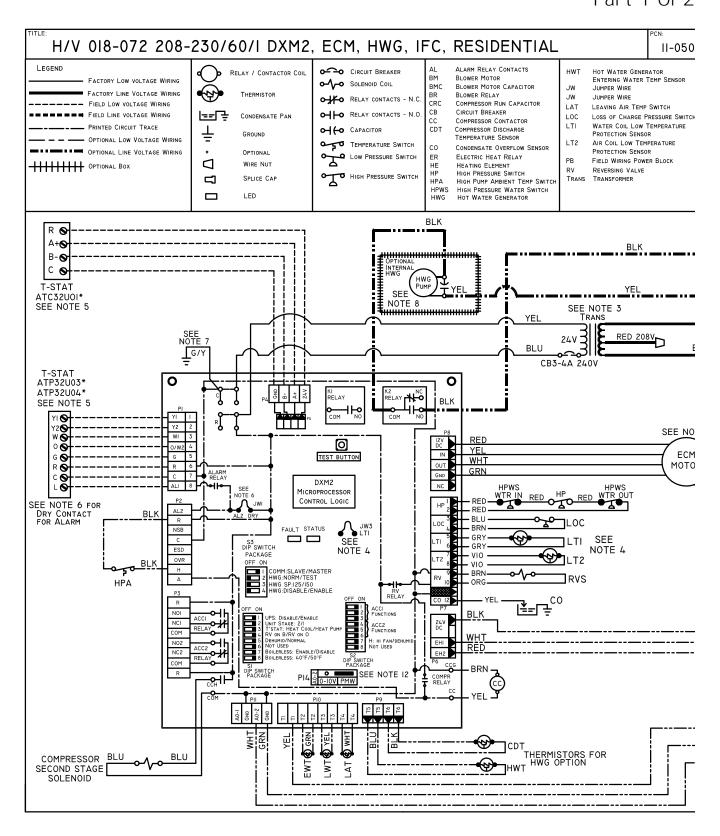
This diagram includes typical wiring details but is not applicable to all units. For specific unit wiring, refer to the diagram or the units' control panel.
