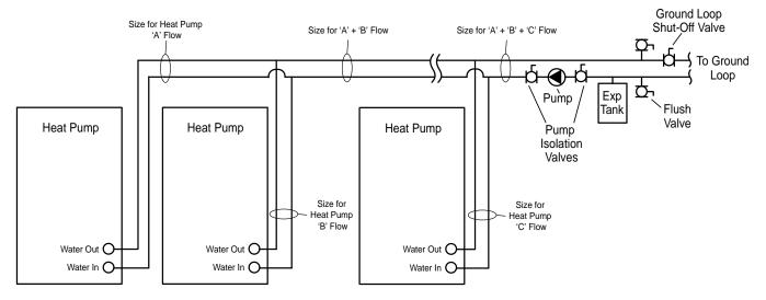
Before flushing, the installer should manually open all modulating valves as detailed in Closed Loop – External Central Pumping section of this manual. Next, flush the ground loop. The installer should close a pump isolation valve and open the ground loop shut-off valve to prevent flow through the indoor loop while flushing the ground loop.
