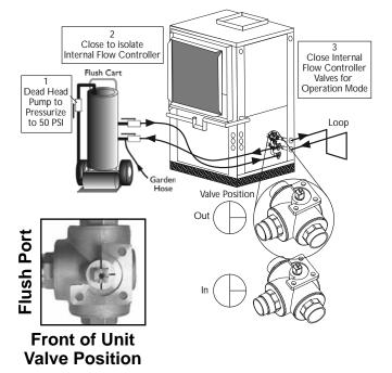
Figure 15e: Valve Position D - Pressurize and Operation
