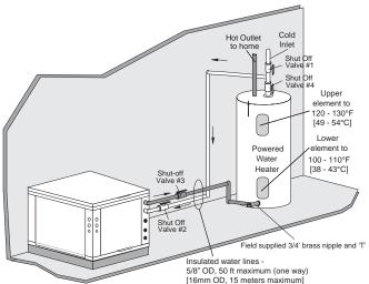
remaining 10 gallons of water from 125°F to 150°F, providing a total of up to 18,743 btu's of heat, or more than twice as much heat as when using the 125°F set point.
