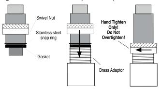
Figure 3: TEP Installation
