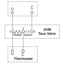
Figure 26: Taco SBV Valve Wiring
