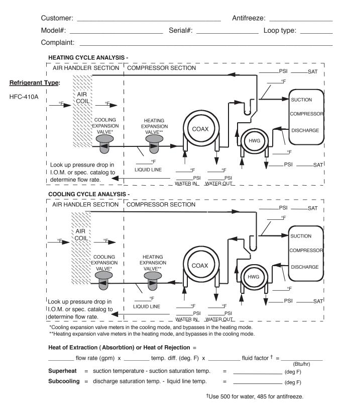
Note: Never connect refrigerant gauges during startup procedures. Conduct water-side analysis using P/T ports to determine water flow and temperature difference. If water-side analysis shows poor performance, refrigerant troubleshooting may be required. Connect refrigerant gauges as a last resort.
