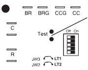
Short test pins together to enter Test Mode and speed-up timing and delays for 20 minutes.
