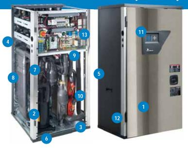
The THW Series offers an extended range refrigeration circuit, capable of ground loop (geothermal) applications as well as open loop (well water) applications. Unique application-specific controls make the THW Series ideal for hydronic heating and domestic hot water generation. The heating-only refrigeration circuit is optimized for high water temperatures, heating efficiencies, and capacities.
