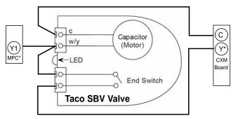
"Valve must be wired in between the CXM and MPC boards. Remove the yellow wire from the CXM board and connect it to the w/y terminal on the valve. Add a new wire from the end switch (bottom connection) to the the Y terminal at the CXM board, and a jumper wire from the w/y terminal to the other side (top connection) of the end switch as shown above.
