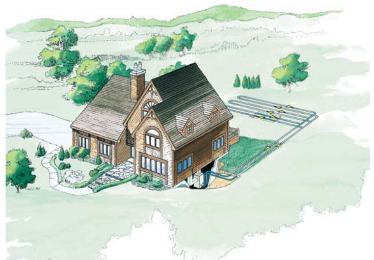
An example of a horizontal loop installation
