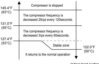
Indoor heat exchange temperature drops
