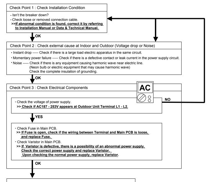
▶ If the symptom does not change by above Check 3, replace Main PCB.
