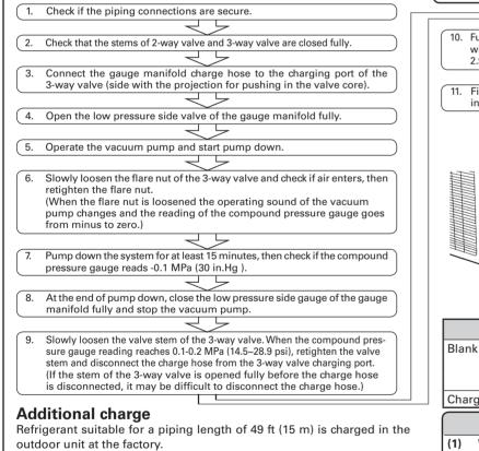
When the piping is longer than 49 ft (15 m), additional charging is necessary. For the additional amount, see the table below.
