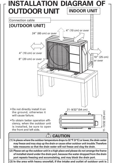
blocked with snow, it might become difficult to get warm and it is likely to because of the breakdown. Please construct a canopy or baffle board.
