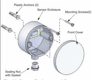
Fig. 25: Sensor Enclosure and Components
