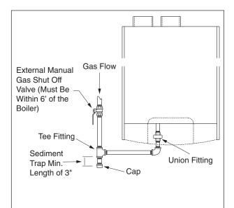
Fig. 16: Recommended Gas Supply Piping
