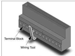
Fig. 19: Using the wiring tool on the terminal blocks
