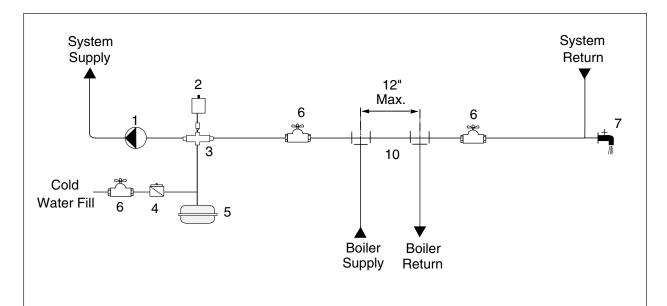
Fig. 6: Near Boiler Piping - Diaphragm Expansion Tank
