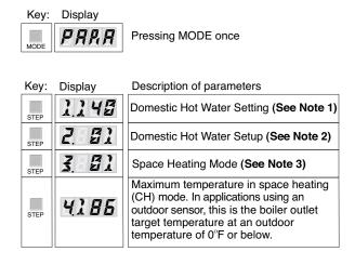
**Note 1:** This parameter is factory set to  $140^{\circ}\text{F}$ . It is important to note the control adds  $46^{\circ}\text{F}$  to this setting, therefore the actual domestic hot water boiler setpoint is  $140^{\circ}\text{F} + 46^{\circ}\text{F} = 186^{\circ}\text{F}$ .
