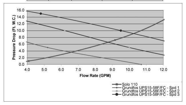
Note: Minimum allowable flow rate at full input: 5 gpm
