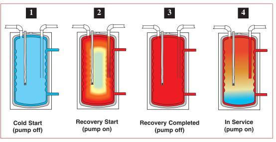
When the thermostat in the inner tank calls for heat, the boiler and circulator start. Boiler water is circulated around the outer tank and heats the domestic water in the inner tank. After transferring its heat, boiler water is returned to the boiler to be re-heated. When the thermostat in the inner tank reaches its pre-set mark, the boiler and circulator shut off.
