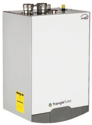
The Prestige Excellence Model Condensing Boiler also incorporates a 14 gallon Indirect Fired Water Heater in the cabinet that is capable of producing 180 gph of domestic hot water.
