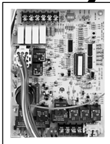
INTEGRATED FURNACE CONTROL
