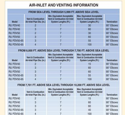
• One 90° elbow is approximately equivalent to 5 feet of pipe.
