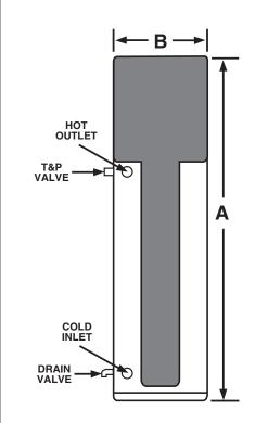
8" TOP CLEARANCE FOR AIR CIRCULATION 3/4" WATER CONNECTIONS 240 VOLT – 1 PH MAX AMP DRAW – 22 AMPS
