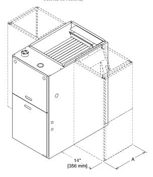
THE RXGR-C24B MUST ONLY BE INSTALLED ON THE SIDE OPPOSITE THE GAS AND ELECTRICAL CONNECTIONS.
