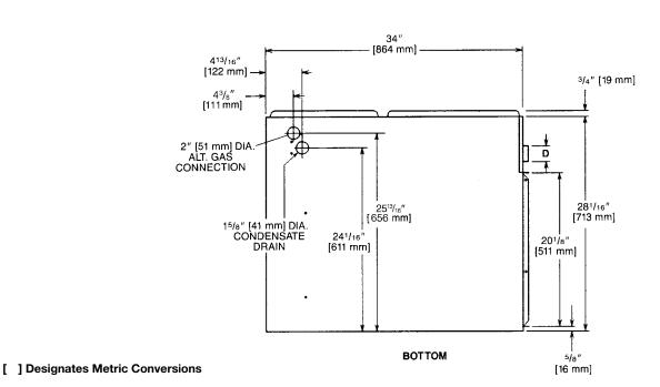
IMPORTANT NOTE: Horizontal furnace may be installed for horizontal left hand air supply ONLY. The condensate trap provided for horizontal application must be installed in the field beneath the unit as directed in the furnace Installation & Operating Instructions.
