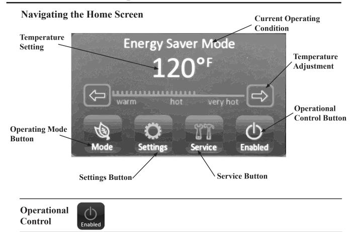
Once power is supplied to the water heater, the Operational Control Buttons can be used to activate the heating of water.
