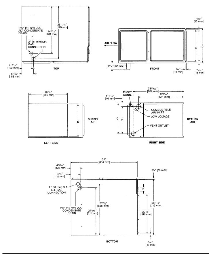
IMPORTANT NOTE: Horizontal furnace may be installed for horizontal left hand air supply ONLY. The condensate trap provided for horizontal application must be installed in the field beneath the unit as directed in the furnace Installation & Operating Instructions.
