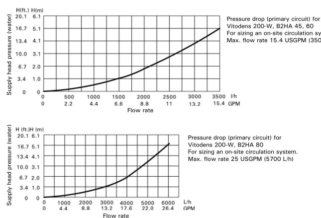
Vitodens 200-W, B2HA 45, 60 For sizing an on-site circulation system. Max. flow rate 15.4 USGPM (3500 L/h)
