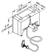
The mixing valve actuator is mounted directly on the Viessmann  $\frac{3}{4}$  to  $2\frac{1}{2}$ " mixing valve.
