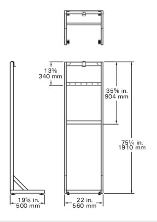
The boiler stand is used for free-standing installation of a single boiler within the mechanical room.
