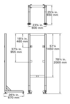
The boiler stand is used for free-standing installation of a single boiler within the mechanical room.
