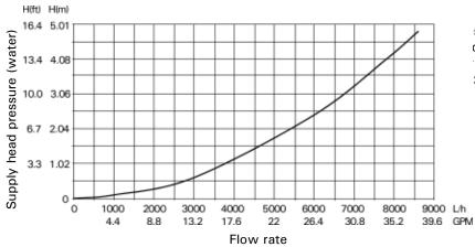
ssure drop (primary circuit) for odens 200-W, B2HA 112, 150 sizing an on-site circulation system. x. flow rate: 38 USGPM (8600 L/h)
