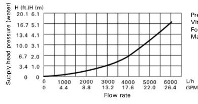
Pressure drop (primary circuit) for Vitodens 200-W, B2HA 100 For sizing an on-site circulation system. Max. flow rate: 25 USGPM (5700 L/h)
