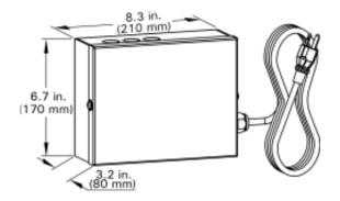
120 VAC Rated voltage: Rated frequency: 60 Hz Rated current: 4 (2) A Power consumption: 4 W
