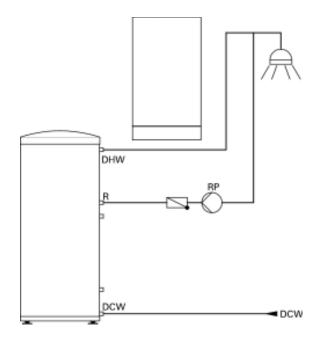
DHW recirculation lines increase the level of comfort and convenience of the domestic hot water supply and reduce water consumption.
