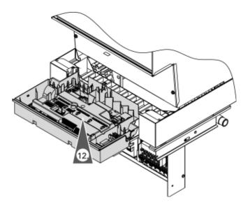
12. Route all connecting cables to the appropriate areas and secure the cables to the control base using existing strain reliefs as shown.
