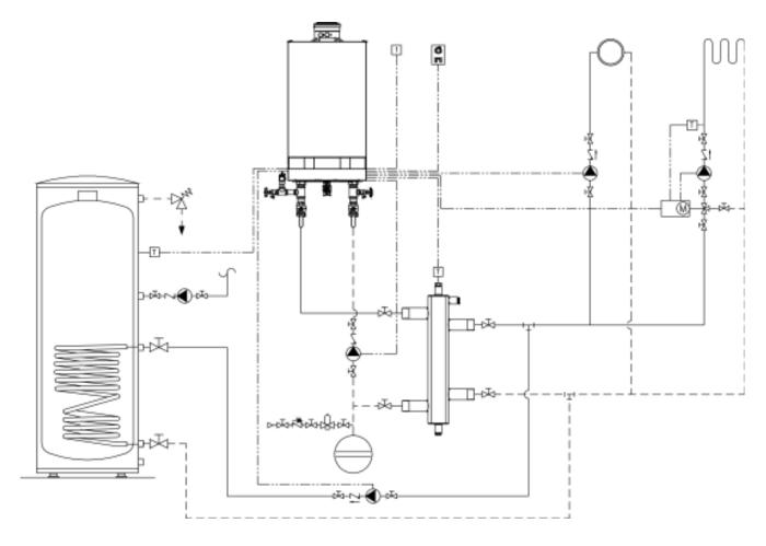
\*Note: When using a low loss header in the system, the DHW connections can be made downstream of the low loss header. See Vitodens 200-W B2HA Service Instructions for applicable system coding information (see coding level 2):
