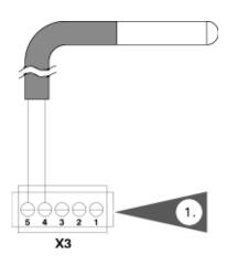
Connect the low-loss header sensor (if used) to terminals X3.4/X3.5 on the boiler control board.
