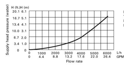
Pressure drop (primary circuit) for Vitodens 200-W, B2HA 80, 100 For sizing an on-site circulation system. Max. flow rate 25 USGPM (5700 L/h)
