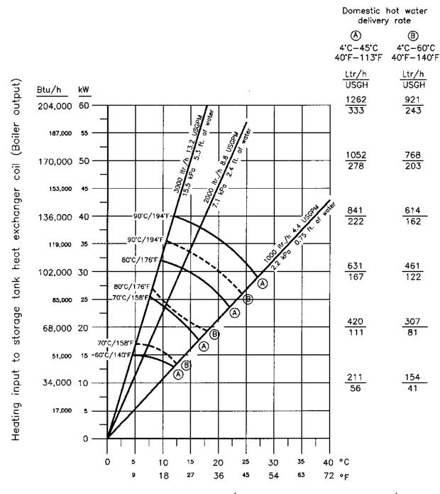
Temperature difference (Boiler supply - Boiler return)
