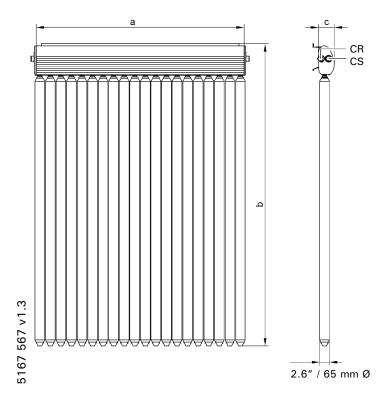
CR Collector return (inlet) CS Collector supply (outlet)
