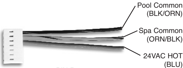
7-PIN Remote Interface Harness
