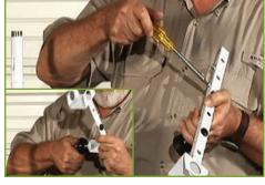
6. Before installing the mounting brackets, make sure to remove the nuts and bolts attached. Now screw the adjustable legs into each bracket.
