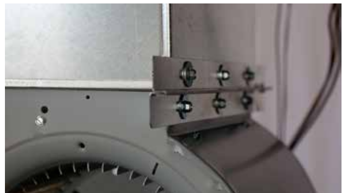
Figure 2: Blower Housing Connections
