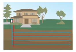
Horizontal Loop: This is the most common loop used when adequate land area is available. Loop installers use excavation equipment such as chain trenchers, backhoes and
