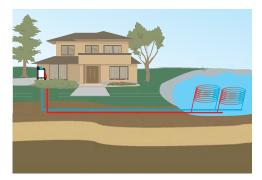
**Pond Loop:** A pond loop is an option if a large body of water is available within approximately 200 feet of the home. A ½ acre, 10 to 12 foot deep body of water is usually adequate to
