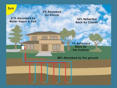
In the summer, this process is reversed in order to cool the home. Heat is drawn from the home, rejected to the loop and absorbed by the earth. The result is a comfortable home all year round.
