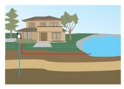
**Open Loop:** This system can be installed if an abundant supply of high quality well water is available. A typical home will require 4 to 8 gallons of water per minute. A proper discharge
