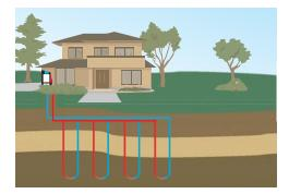
Vertical Loop: This loop is used mainly when land area is limited and in retrofit applications of existing homes. A drilling rig is used to bore holes at of depth of 150 to 300 feet per ton. A
