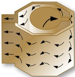
Thermo Pride's revolutionary Octatherm design forces flue gases into a high rate of agitation as they pass through the heat exchanger. This increases heat transfer and efficiency, resulting in more uniform surface heating.
