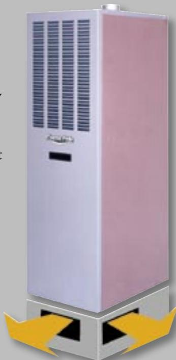
Additional rooms may be heated by connecting ductwork to the base, and then through the wall to adjacent rooms. No ductwork, grilles, or cutouts are provided with the base. The installer will cut the base as needed.
