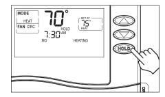
**Press** to permanently hold the temperature at its current setting. This will override the temperature settings for all time periods of the programmed schedule. With the thermostat in permanent override, the thermostat temperature can be manually adjusted and will stay at that setting until the override is cancelled.
