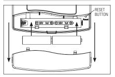
The thermostat can either be AC or battery powered, or both. When wired to be AC powered, the batteries are optional and only provide backup power to the clock.
