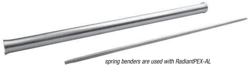
spring benders are used with RadiantPEX-AL tubing to prevent over bending and kinking of the tubing. spring benders are not needed for RadiantPEX.
