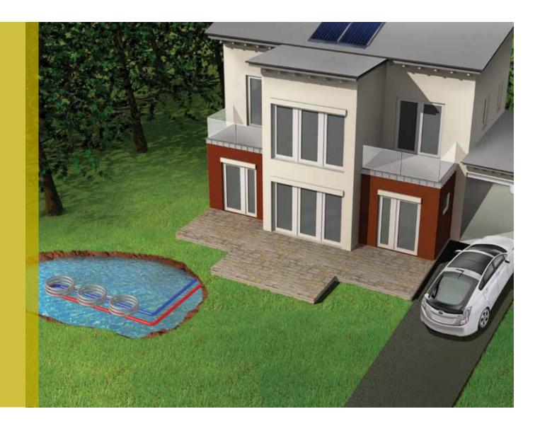
This type of design is economical when a project is located near a body of water. Fluid circulates through polyethylene piping in a closed system, just as it does through ground loops but in this case underwater. The pipes may be coiled in a slinky to fit more surfaces into a given amount of space. The lake needs to be a minimum size and depth depending on the load. Lake loops have no adverse impact on the aquatic system.
