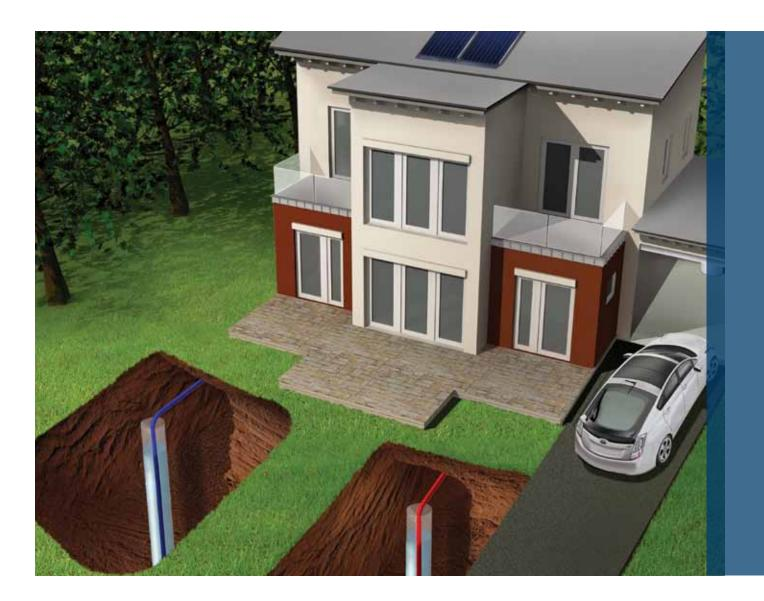
This type of design is only possible if there is sufficient ground water available in a well, a lake or river in the area. The water must be of good quality. Local codes may limit the use of this system in certain areas. The system is open which means that water is pumped directly into the geothermal unit and then discharged either into a return well or a body of water. The water quality remains unaffected.
