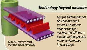
Unique MicroChannel Coil construction creates a superior heat exchange surface that allows a smaller unit to provide more performance in less space
