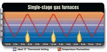
Traditional single-stage gas furnaces operate much like a light bulb—either on or off. This can create wide and uncomfortable temperature fluctuations in your home.
