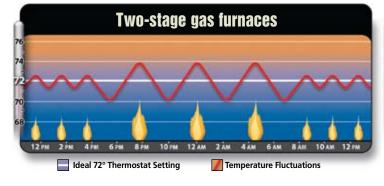
Two-stage gas furnaces offer an intermediate level of performance. Operation varies between first and second stage based on demand. However, indoor temperature levels still fluctuate, relative to your thermostat setting.
