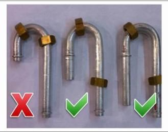
Tighten the nut that connects the gas tube to both the Gas Valve and the Fan Motor with 10" crescent wrench. Do not over tighten or you will damage the aluminum gas tube. Turn on all water, gas and electrical to unit and test ignition.
